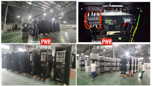
30 × 120/180 kW PV control cabinets
